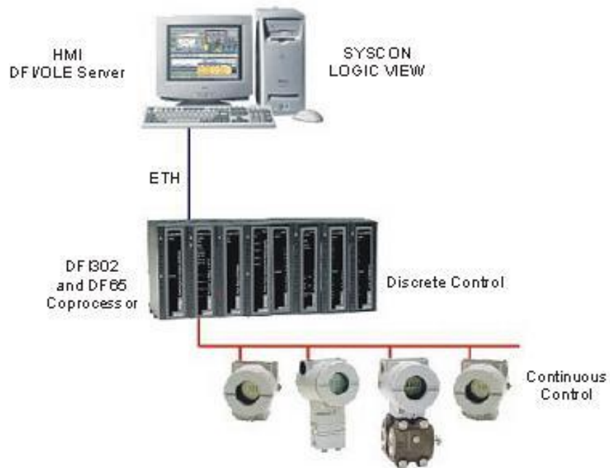
Figure 18. 1 - DFI302 System and Co-processor
