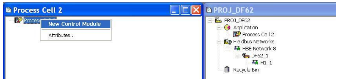
Figure 19.25 – Creating the New Control Module
