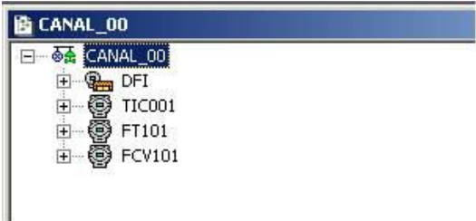
Figure 16. 14 – Device added into the Fieldbus channel
