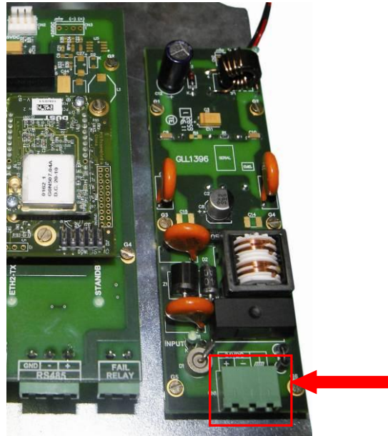
Figure 2.59 – Power supply connector
