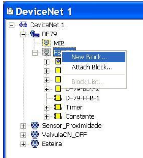
Figure 21. 39 – Inserting new function blocks to the device
