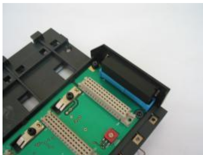
Figure 2.11 - DF2 terminator installed
