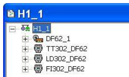
Figure 19. 17 – Devices added into the Fieldbus channel
