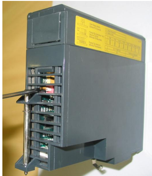
Figure 18. 10 – Locating the DF65 Rotary Switch
