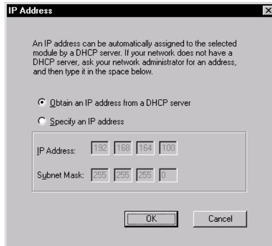
18 - The default option is to obtain the IP address from DHCP Server. Click the **Specify an IP address** option.
