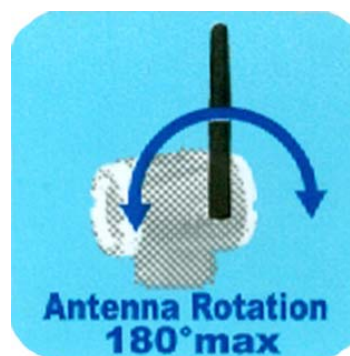
Figure 1.8 – Antenna rotation limits
