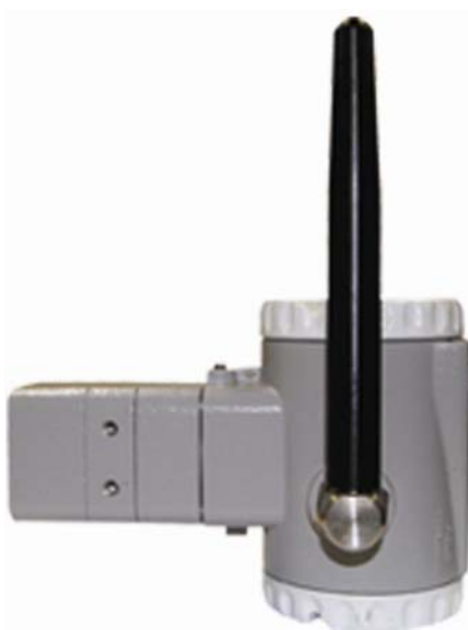
Figure 1.9 – Correct position of the antenna with device horizontally
