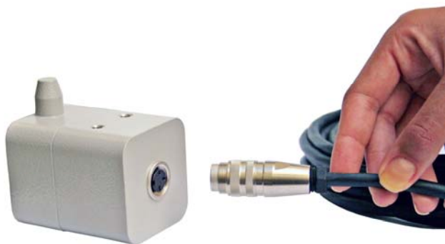
Figure 1.14 - Connecting the Cable to the Remote Position Sensor
