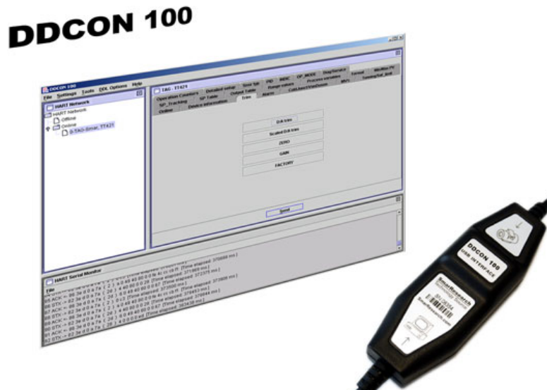
Figure 3.9 – DDCON 100 - DDL Based HART Configurator
