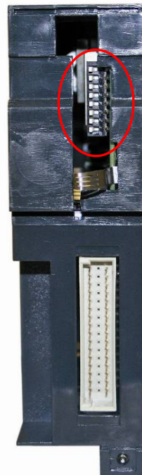
Figure 17 – Switches 1 to 8 for communication rate adjustment
