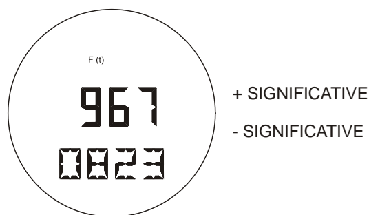
Figure 4.5 – Typical Monitoring Mode Display Showing the Total, in this case 19.6708.23
