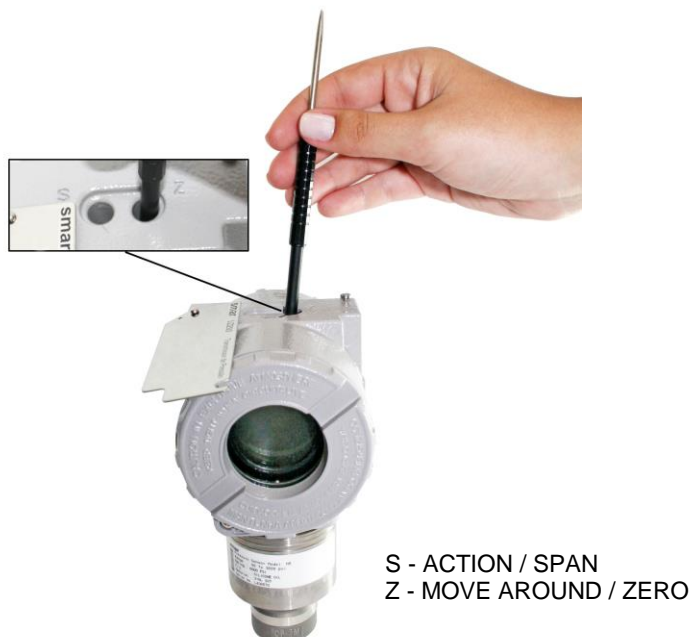
Figure 3.31 - Local Adjustment Holes
