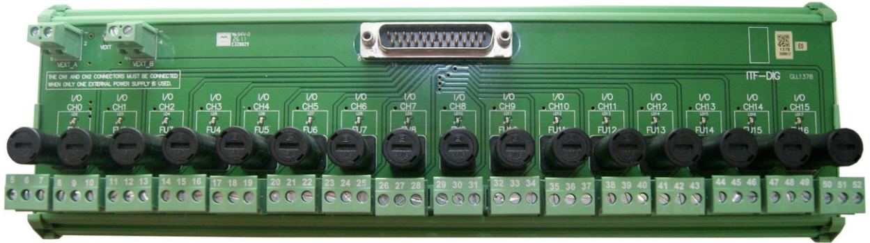
Figure 25 – ITF-DIG Interface for Panel
