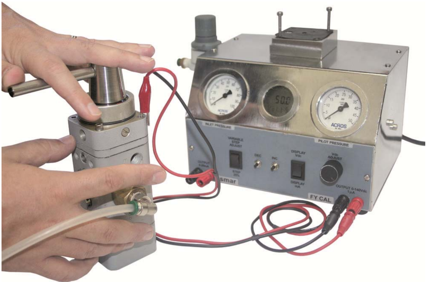
Figure 12 - Piezo Base Calibration on the block with help the Base Tool Calibration
