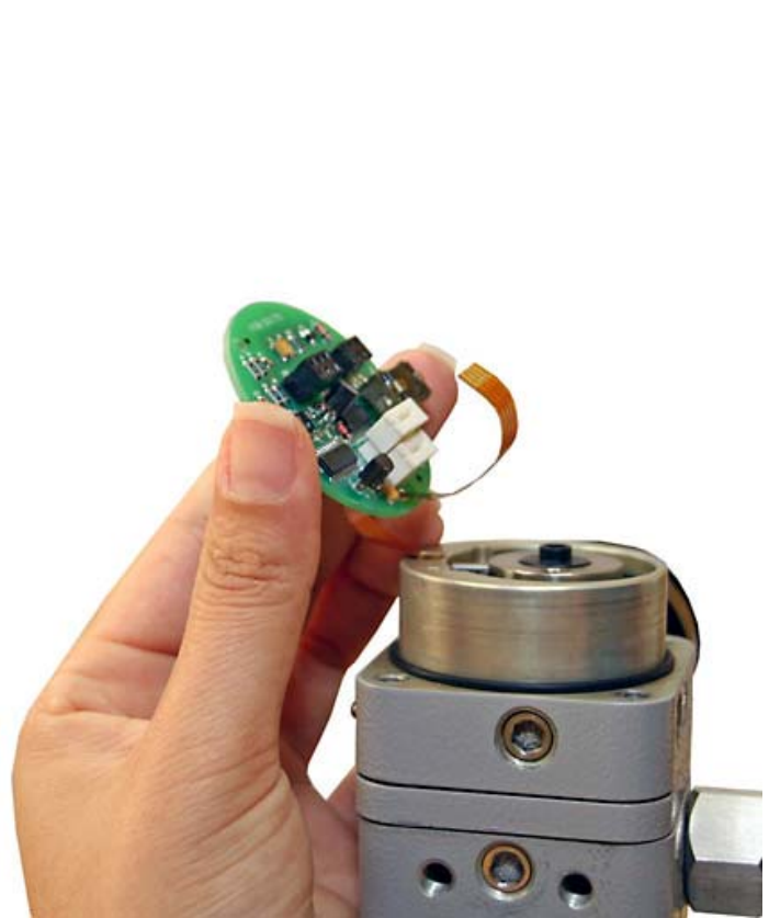
Figure 6.12 - Flat Cable loosened from the connector
