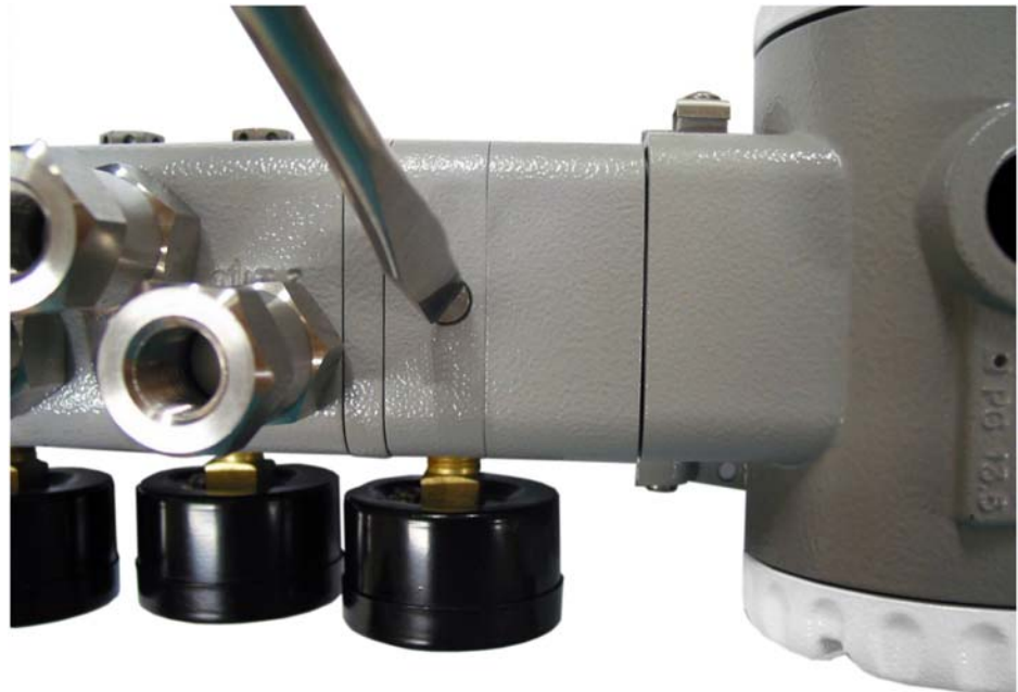
Figure 6.15 – Removing the Restriction Screw
