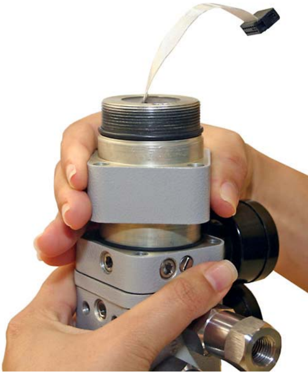
Figure 6.7 – Loosening the Assembled Base Connection Cover
