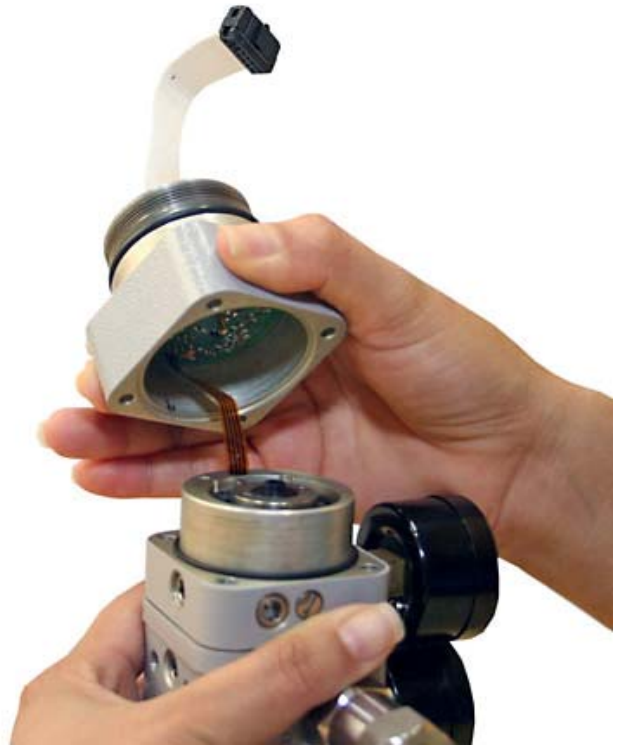
Figure 6.8 – Loosened Connection Cover
