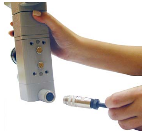
Figure 1.16 - Connecting the Cable to the Positioner
