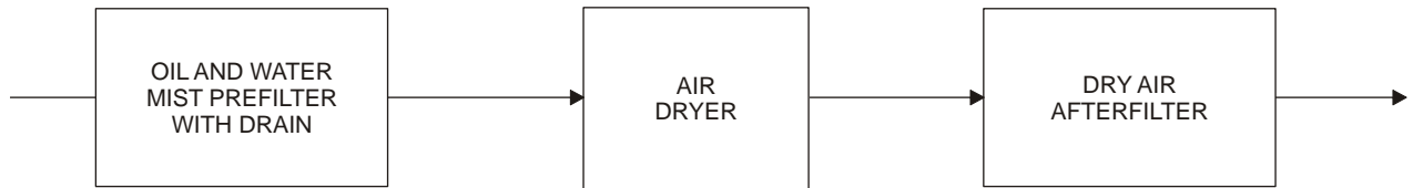
Figure 1.10 - Air Quality Conditioning System
