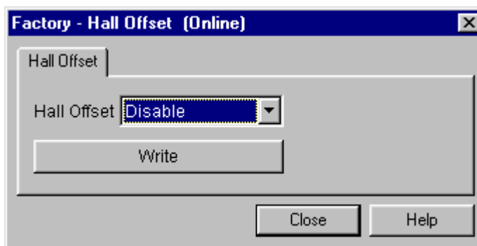
Figure 3.32 - Disabling the Hall's Offset Compensation
