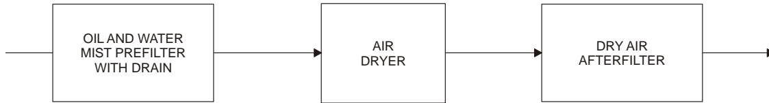
Figure 1.10 - Air Quality Conditioning System
