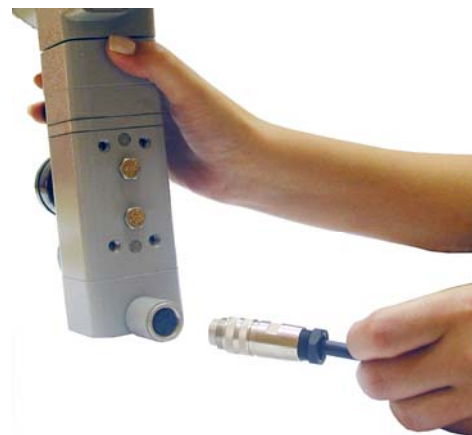
Figure 1.16 - Connecting the Cable to the Positioner
