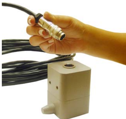
Figure 1.15 - Connecting the Cable to the Remote Hall Sensor
