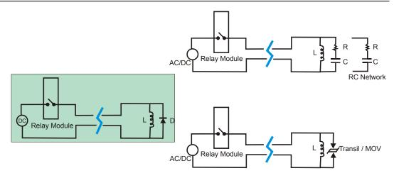
Figure 1.6 - Filters for AC and DC loads
