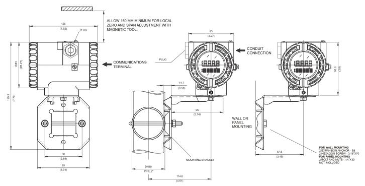
Figure 1.1 - Dimensional Drawing and Mounting Positions
