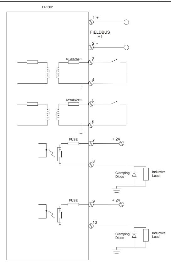
Figure 1.4 – Example of Output and Input Connections
