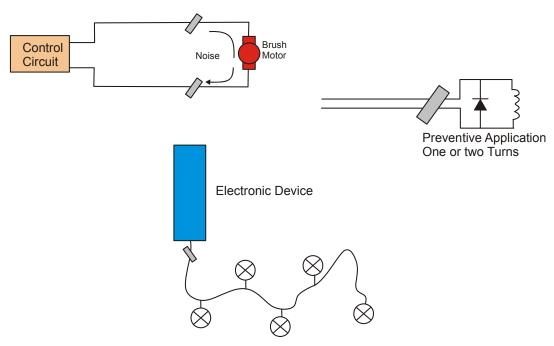
Figure 1.9 – Ferrite Application on Control Lines
