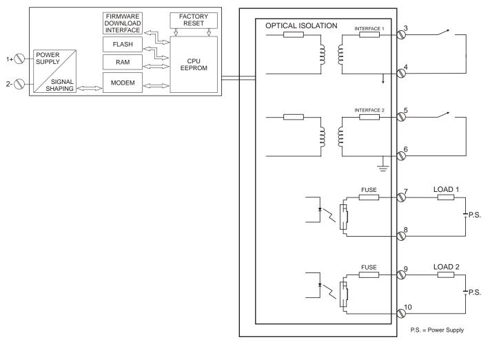
Figure 2.1 – FRI302 Block Diagram
