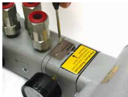
Figure 5.19 - Remove the Transducer Serial Number Plate
