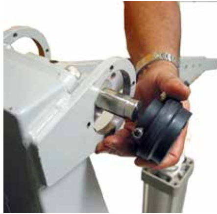
Figure 1.18 - Placing the Magnet
