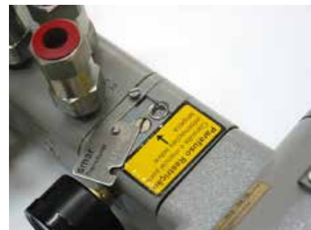
Figure 5.20 - Transducer Serial Number Plate Removed
