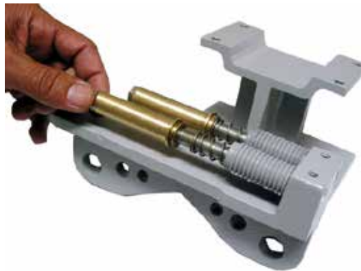
Figure 5.15 - Disassembling Spring and Below Set
