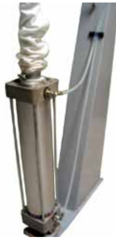
Figure 1.29 - Detail of the Pipe Installed on the Rotary ACP for Air Supply
