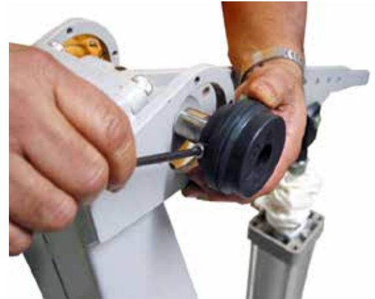
Figure 1.19 – Fixing the Screw (Do not tight it)
