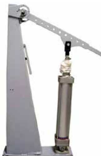
Figure 1.15 – Rotary ACP Base with the Cylinder Installed
