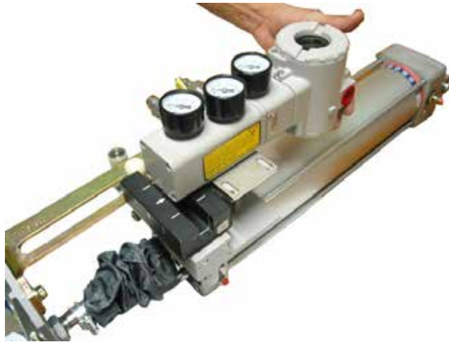
Figure 5.2 - Disassembling the Positioner of the Cylinder
