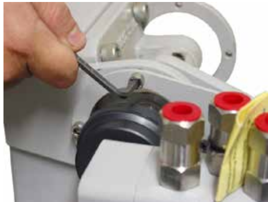
Figure 1.22 - Positioner and Bracket Installed into the ACP Base
