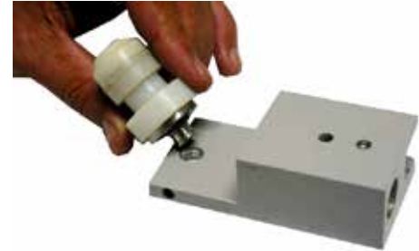
Figure 5.14 - Disassembling the mobile roller
