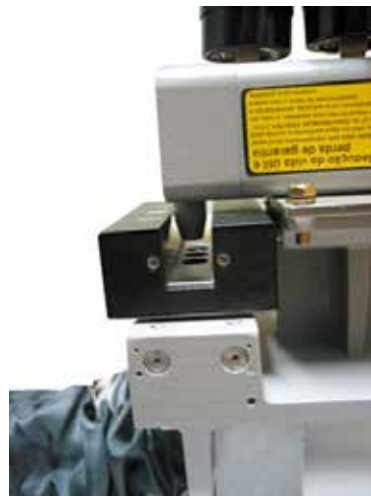
Figure 1.13 – Magnet Alignment with the Hall Sensor
