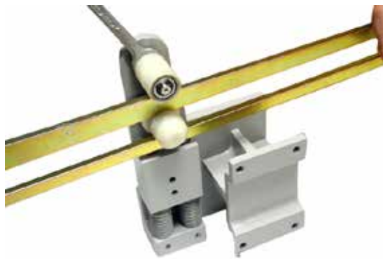
Figure 5.9 - Disassembling the Fixed Roller
