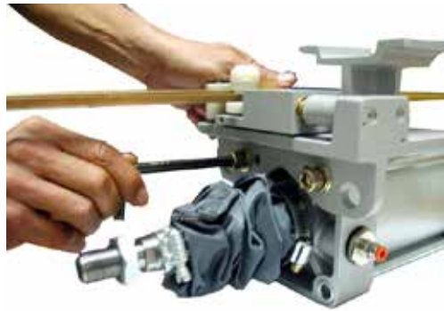
Figure 5.7 - Disassembling the FY301 Positioner Bracket
