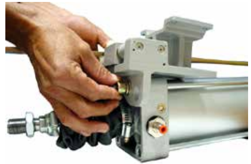
Figure 5.8 - Unfasten the Allen Screws
