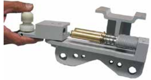
Figure 5.12 - Disassembling the Mobile Base Sub Set
