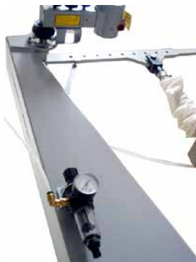
Figure 1.30 - Installing the Air Filter
